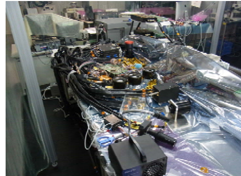
Fig. 12. Flight model functional test of ChubuSat-1
