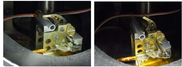
Fig. 9. Receiving antenna hold and release mechanism of ChubuSat-1
